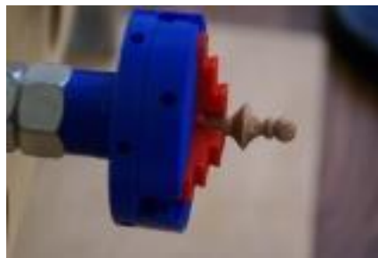
Top mounted in Regular Jaws
